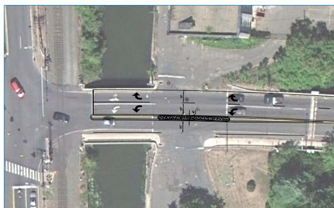
Possible Mitigation: Median Barrier at Ahlstrom Driveway
